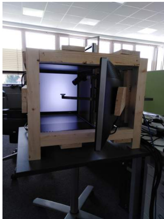
Figure 3.1: Photo of the final lightstage. The door is opened to see the object holder and the camera inside.
